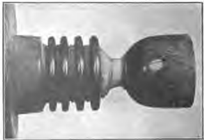
Fig. 119. Goblet Rings Polished.
